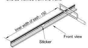
If the distance between the cutting face of the rail and the reference mounting hole is no less than 80mm, make a new hole \$\phi 5.5mm\$ for installing the rail at the position 50mm from the end.
