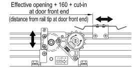
When the clutch gear is inserted or remoned, be sure to turn it as following instruction
