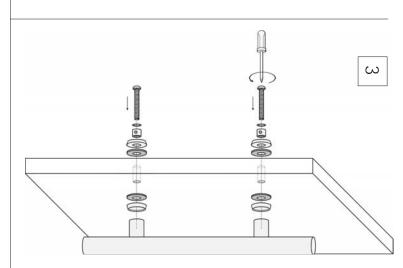
3-2. Mount the outer handle on the door along with rubber washers, end caps, fixing
