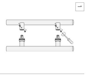
Unscrew 4 x M4 screws by screwdriver.
