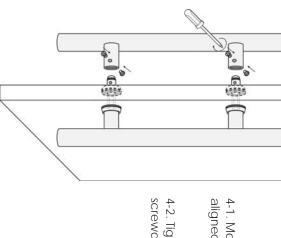
4-1. Mount the inner handle aligned to the outer handle.
