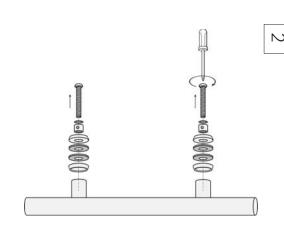
Loosen 2 x M8 center bolts by screwdriver.
