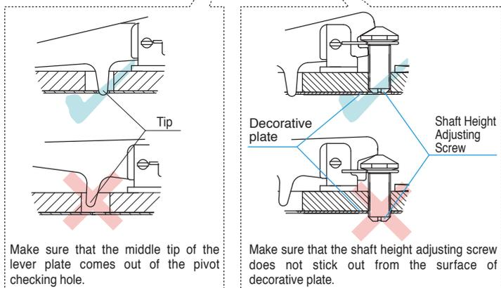
\*Same for the reverse pivot installation. Make sure that the middle tip of the lever plate comes out properly.
