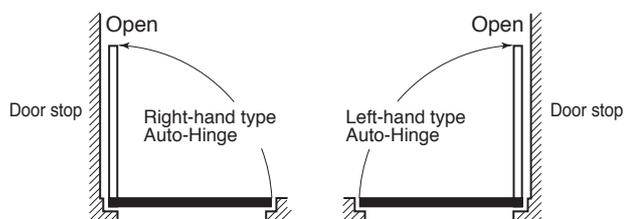
● When using for the smoke ventilations or air intake doors (automatic opening), use the Auto-Hinge left and right opposite. Also use the U-2NH receptive base.
