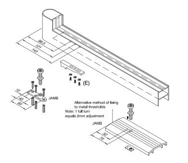
Prepare the bottom rail of the door to accomodate the pivot shoe with 2No. drilled and tapped M6 holes at 98.5mm and 143mm centres.
