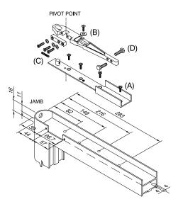
Prepare the top rail of the door as detailed, ensuring that the internal faces of the stile and top rail have been cut away to enable the closer spindle to be engaged during door hanging. Drill 7mm hole in the heel of the door giving access to the adjustment screw (C). Fit steel arm channel to the door top rail using the 4No. M6 csk screws (A).
