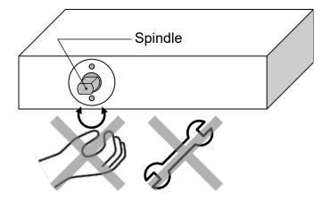
Do NOT rotate the spindle (pivot pin of closer main unit) by hand or tools.
